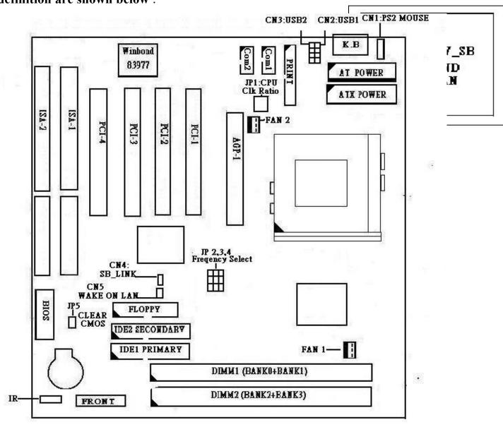
2.7 USB Connector (Right: USB1, Left: USB2): CN2/CN3
