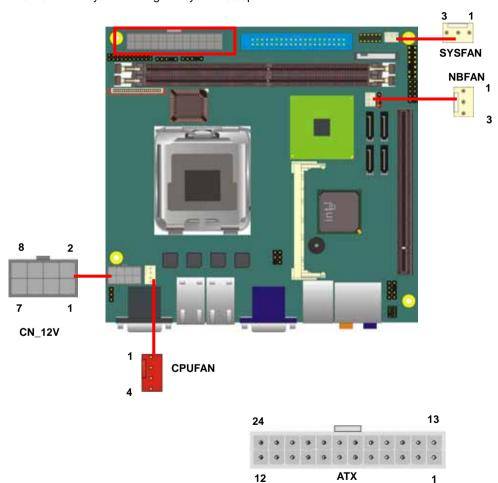
Connector: **ATX** Type: 24-pin ATX power connector
