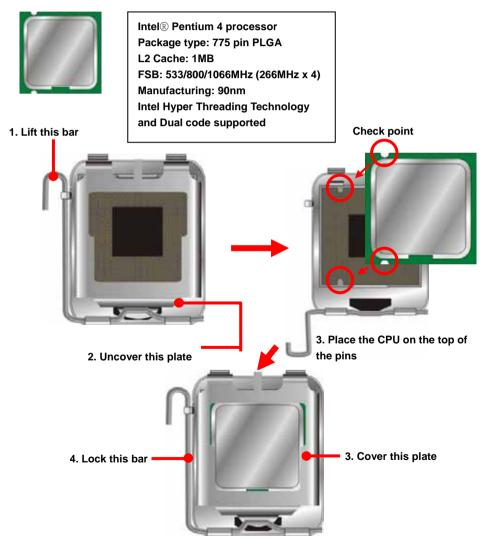
Notice: Please place the CPU on the pins tenderly to avoid bending the pins
