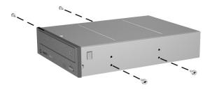
2. Position the guide screws on the drive into the J-slots in the drive bay **●**. Then, slide the drive towards the rear of the workstation **②**.
