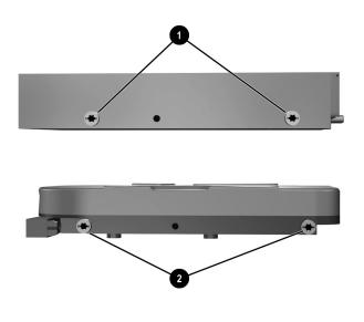
The guide screws on a 3.5-inch diskette drive ① are placed closer together than on the hard drive ②.
