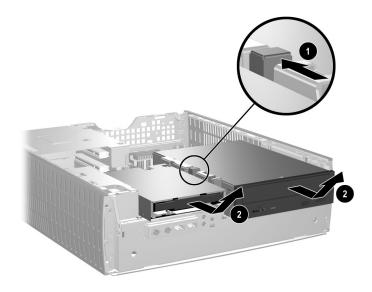
When replacing the drive, transfer the four screws from the old drive to the new one. The screws take the place of drive rails. You will need a Torx T-15 screwdriver to remove and re-install the guide screws.
