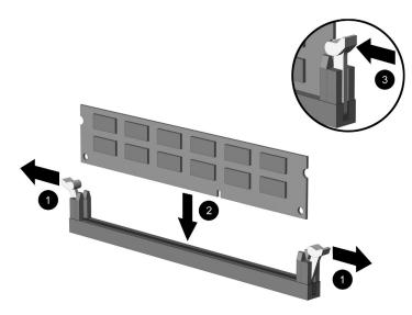
A memory module can be installed in only one way. Match the notch on the module with the tab on the memory socket.
