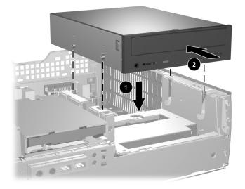
The drive release latch automatically locks in place when installing a drive.
