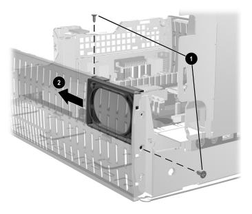
To install the speaker, reverse the removal procedures.
