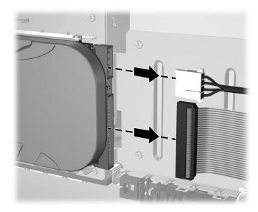
Disconnecting Cables from the Hard Drive
