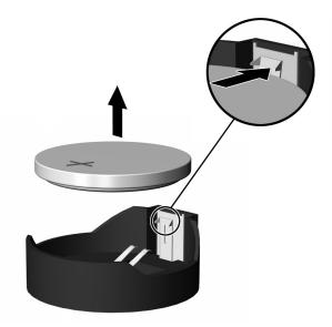
3. To insert the new battery, slide one edge of the replacement battery under the holder's lip with the positive side up. Push the other edge down until the clamp snaps over the other edge of the battery.
