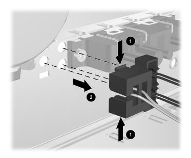
To install the power switch assembly, reverse the removal procedure.
