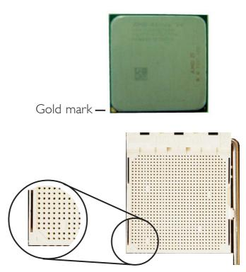
6. Insert the CPU into the socket until it is seated in place. The CPU will fit in only one orientation and can easily be inserted without exerting any force.
