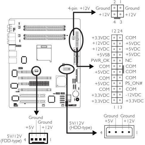
Use a power supply that complies with the ATX12V Power Supply Design Guide Version 1.1. An ATX12V power supply has a standard 24-pin ATX main power connector and a 4-pin +12V power connector that must be inserted onto CN10 and CN9 connectors respectively.
