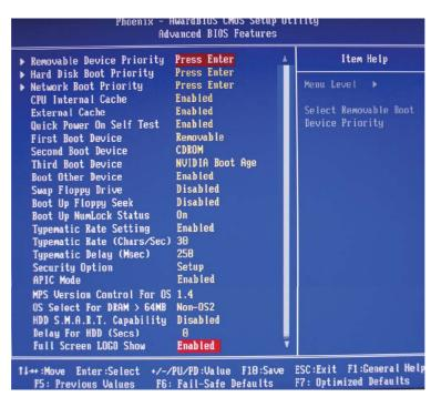
The screen above list all the fields available in the Advanced BIOS Features submenu, for ease of reference in this manual. In the actual CMOS setup, you have to use the scroll bar to view the fields. The settings on the screen are for reference only. Your version may not be identical to this one.
