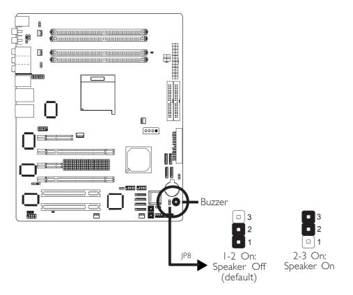
The system board is equipped with a buzzer which serves as the PC's speaker. By default the buzzer is "on" allowing you to hear the system's beep messages and warnings. If you intend to use an external speaker, turn this function off by setting JP8 pins I and 2 to On.
