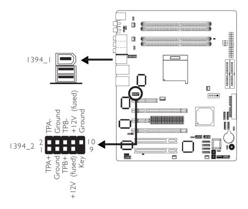
The system board is equipped with an onboard IEEE 1394 port at location CN3 (IEEE 1394\_1) of the system board.
