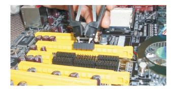
In order for the jumper cap to come off from the hook, slightly open the arms of the clipper.
