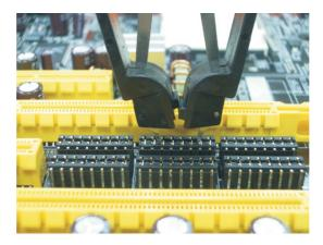
This will easily remove the jumper cap.
