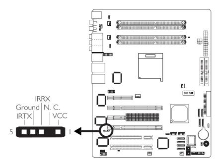
Connect the cable connector from the IrDA module to the IrDA connector (J5).
