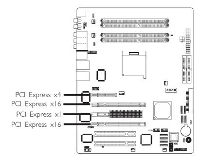
Install PCI Express x16 graphics card, that comply to the PCI Express specifications, into the PCI Express x16 slot. For "SLI" models which support the NVIDIA SLI technology, refer to the next section (SLI Technology) for more information.
