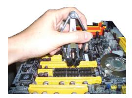
Insert the hooks of the clipper into the jumper cap. Grip the clipper firmly, but not exerting pressure, then pull it upward.
