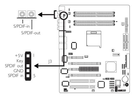
The system board is equipped with an onboard S/PDIF-in RCA jack (red) and a S/PDIF-out RCA jack (yellow) at locations CN5 and CN7 respectively.
