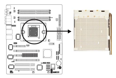
4. Unlock the socket by pushing the lever sideways, away from the socket, then lifting it up to a 90° angle. Make sure the lever is lifted to at least this angle otherwise the CPU will not fit in properly.
