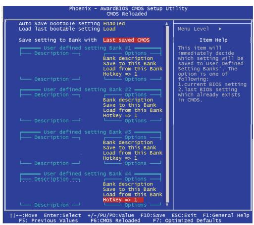
The screen above list all the fields available in the CMOS Reloaded submenu, for ease of reference in this manual. In the actual CMOS setup, you have to use the scroll bar to view the fields. The settings on the screen are for reference only. Your version may not be identical to this one.
