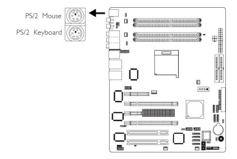
The system board is equipped with an onboard PS/2 mouse (Green) and PS/2 keyboard (Purple) ports - both at location CN2 of the system board. The PS/2 mouse port uses IRQ12. If a mouse is not connected to this port, the system will reserve IRQ12 for other expansion cards.
