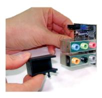
2. Align the module's plugs above the mounting holes then insert the plugs from the top through to the bottom of the system board. While at it, the 14-pin connector at the solder side of the module must also insert into the Karajan audio connector at location J7 of the system board. Make sure the plugs snap firmly out the bottom of the board.
