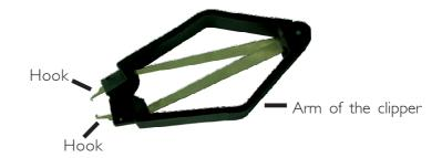
Position the clipper above the jumper cap. Handle the clipper as shown in the illustration below. Handling it this way will prevent exerting too much pressure that might cause breaking the arms of the clipper.
