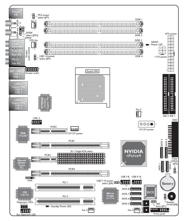
SLI / Single VGA Select jumper - for ''SLI'' models only. Silicon Image Sil3114 and SATA 5 to SATA 8 - for ''DR'' models only. Diagnostic LED connector - for LANPARTY nF4 SLI-DR only.
