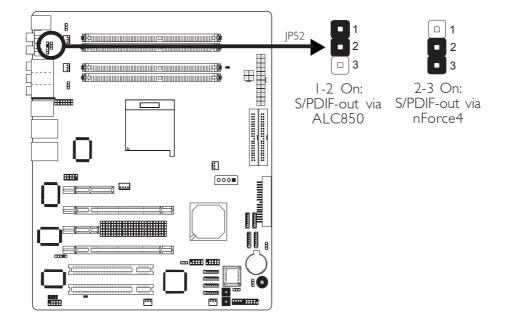
JP52 is used to select the controller that will send signal to the S/PDIF-out port.
