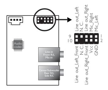
Remove the jumper caps from pins 5-6 and pins 9-10 of J4 prior to connecting the front audio cable connector. Make sure pin 1 of the cable connector is aligned with pin 1 of J4. If you are not using this connector, make sure to replace the jumper caps back to their original pin locations.
