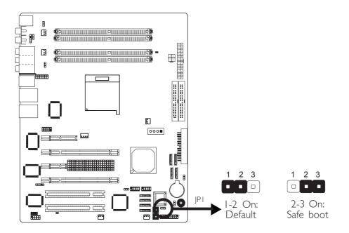
JP1 is used to safely reboot the system whenever the system hangs and you are unable to restart the system.
