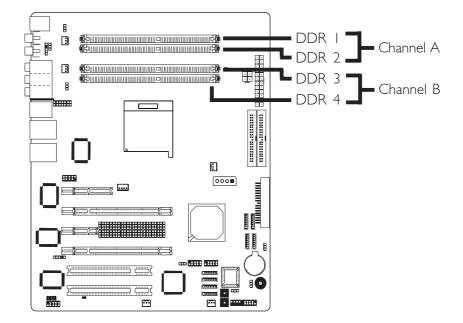
The system board supports DDR SDRAM DIMM. Double Data Rate SDRAM (DDR SDRAM) is a type of SDRAM that doubles the data rate through reading and writing at both the rising and falling edge of each clock. This effectively doubles the speed of operation therefore doubling the speed of data transfer.
