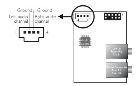
The CD-in (J2) connector on the Karajan audio module is used to receive audio from a CD-ROM drive, TV tuner or MPEG card.
