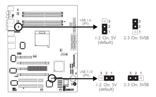
JP5 and JP6 are used to select the power of the USB ports. Selecting 5VSB will allow you to use the USB keyboard or USB mouse to wake up the system..
