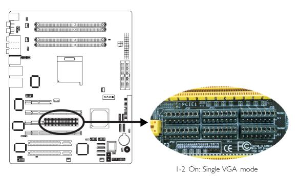
The illustration below shows the bandwidth of the PCI Express slots when set in Single VGA mode.
