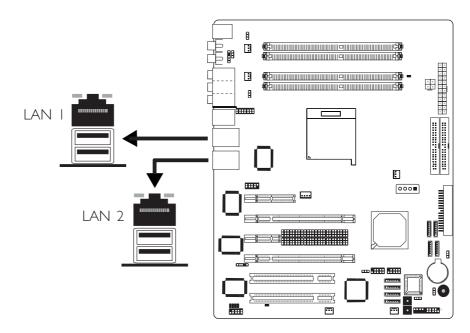
The system board is equipped with 2 onboard RJ45 LAN ports. LAN I which is controlled by the Vitesse VSC8201 Gigabit Phy chip is at location CN4 and LAN 2 which is controlled by the Marvell 88E8001 Gigabit PCI chip is at location CN6.
