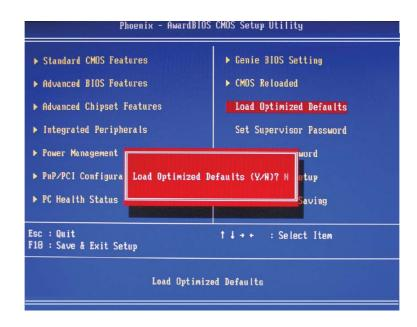
Type <Y> and press <Enter> to load the Setup default values.
