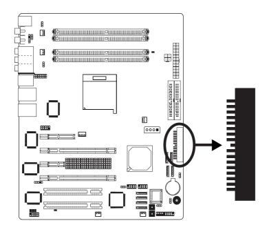
The system board is equipped with a 90° floppy disk drive connector that supports two standard floppy disk drives. To prevent improper floppy cable installation, the floppy disk header has a keying mechanism. The 34-pin connector on the floppy cable can be placed into the header only if pin 1 of the connector is aligned with pin 1 of the header.
