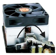
6. Connect the CPU fan's cable connector to the CPU fan connector on the system board.
