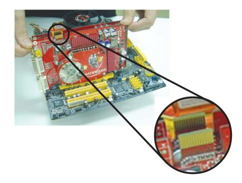
8. Align the SLI bridge (included in the system board package) above the SLI connector of the graphics cards then insert the bridge until it is properly seated in place.
