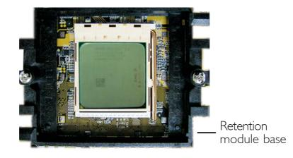
3. Place the heat sink on top of the CPU. Now hook one side of the retention clip onto the retention module base by fitting the holes on the retention clip into the retaining tabs of the retention module base.
