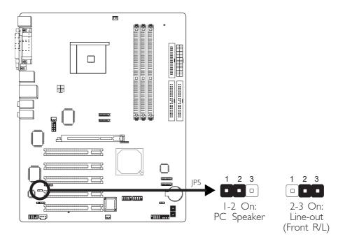
JP5 is used to select the system's beep messages and warnings to come from the line-out (front R/L) jack or the PC speaker.
