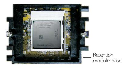
3. Place the heat sink on top of the CPU. Now hook one side of the retention clip onto the retention module base by fitting the holes on the retention clip into the retaining tabs of the retention module base.
