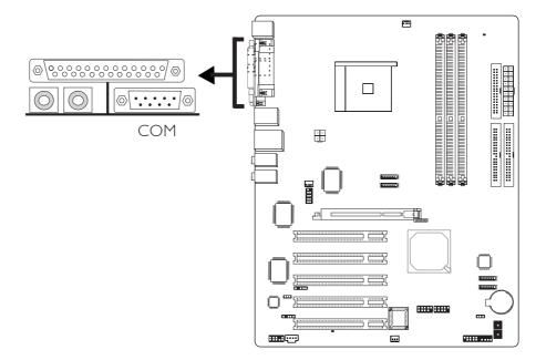
The system board is equipped with an onboard serial port (Teal/ Turquoise) at location JI. The serial port is an RS-232C asynchronous communication port with 16C550A-compatible UARTs that can be used with a modern, serial printer, remote display terminal or other serial devices.
