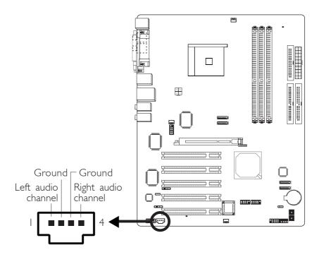
The CD-in (J4) connector is used to receive audio from a CD-ROM drive, TV tuner or MPEG card.
