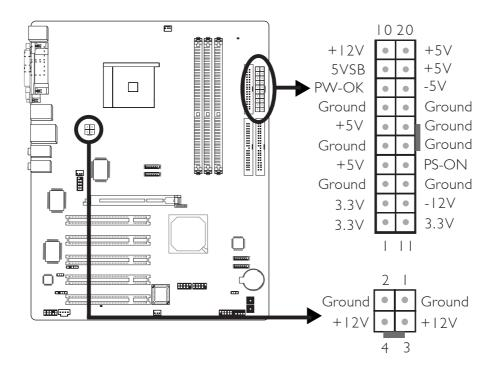
Use a power supply that complies with the ATX12V Power Supply Design Guide Version 1.1. An ATX12V power supply has a standard 20-pin ATX main power connector and a 4-pin +12V power connector that must be inserted onto J24 and CN9 connectors respectively.
