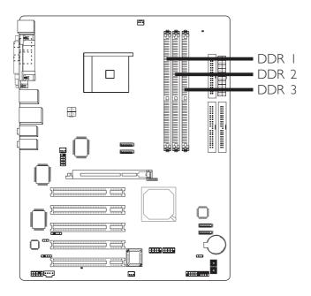
The system board supports DDR SDRAM DIMM. Double Data Rate SDRAM (DDR SDRAM) is a type of SDRAM that doubles the data rate through reading and writing at both the rising and falling edge of each clock. This effectively doubles the speed of operation therefore doubling the speed of data transfer. Refer to chapter I (System Memory section) for detailed specification of the memory supported by the system board.
