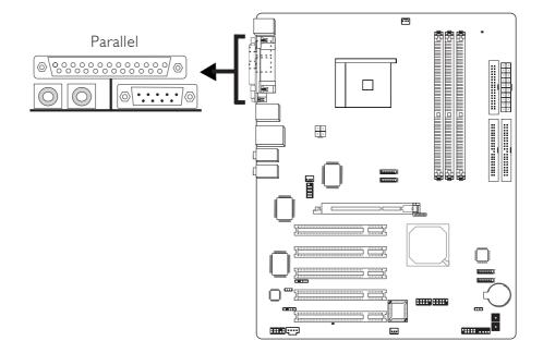
The system board has a standard parallel port (Burgundy) at location CN1 for interfacing your PC to a parallel printer. It supports SPP, ECP and EPP.
