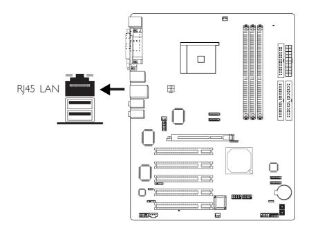
The system board is equipped with an onboard RJ45 fast-ethernet LAN port at location CN4 of the system board. It allows the system board to connect to a local area network by means of a network hub.
