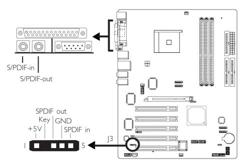
The system board is equipped with an onboard S/PDIF-in RCA jack (red) and a S/PDIF-out RCA jack (yellow) at locations CN5 and CN7 respectively.
