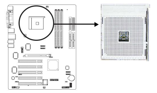
4. Unlock the socket by pushing the lever sideways, away from the socket, then lifting it up to a 90° angle. Make sure the lever is lifted to at least this angle otherwise the CPU will not fit in properly.
