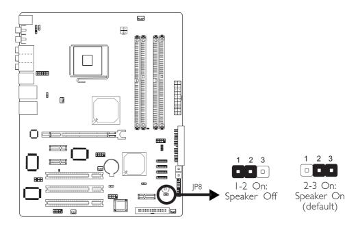
JP8 is used to turn on or off the PC's speaker. Turning on the speaker will allow you to hear the system's beep messages and warnings.
