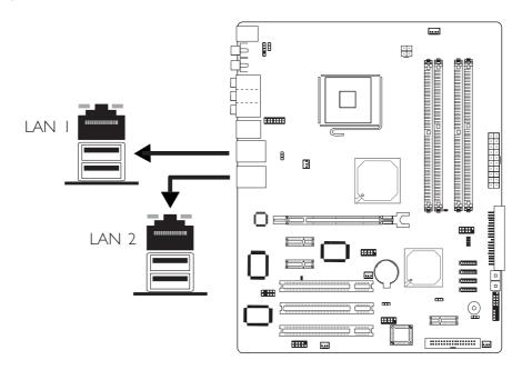
The system board is equipped with 2 onboard RJ45 LAN ports. LAN I which is controlled by the Marvell 88E8053 PCI Express controller is at location CN7 and LAN 2 which is controlled by the Marvell 88E8001 PCI chip is at location CN12.
