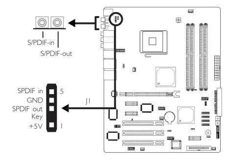
The system board is equipped with an onboard S/PDIF-in RCA jack (red) and a S/PDIF-out RCA jack (yellow) at locations CN4 and CN5 respectively.
