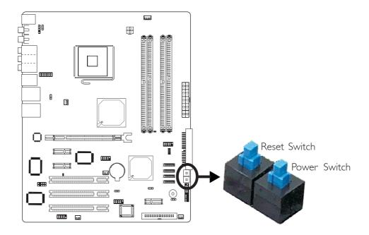
The presence of the power switch and reset switch on the system board are user-friendly especially to DIY users. They provide convenience in powering on and/or resetting the system while fine tuning the system board before it is installed into the system chassis.
