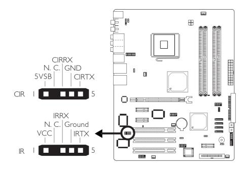
Connect the cable connector from your CIR/IR module to the CIR connector (J24) or IR connector (J8).
