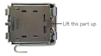
6. Unlock the socket by pushing the lever down, moving it away from the side tab of the socket, then lifting it up.
