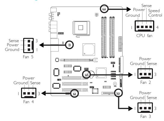
Connect the CPU fan's cable connector to the CPU fan connector (J21) on the system board. Fan 2 (J19), Fan 3 (J20), Fan 4 (J22) and Fan 5 (J23) are used to connect additional cooling fans. The cooling fans will provide adequate airflow throughout the chassis to prevent overheating the CPU and system board components.
