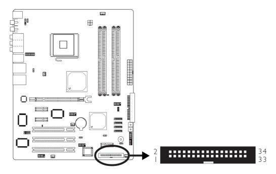
The system board is equipped with a shrouded floppy disk drive connector that supports two standard floppy disk drives. To prevent improper floppy cable installation, the shrouded floppy disk header has a keying mechanism. The 34-pin connector on the floppy cable can be placed into the header only if pin 1 of the connector is aligned with pin 1 of the header.
