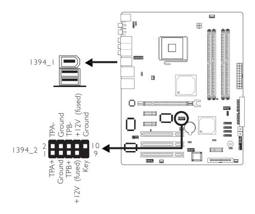
The system board is equipped with an onboard IEEE 1394 port at location CN8 (IEEE 1394\_I) of the system board.
