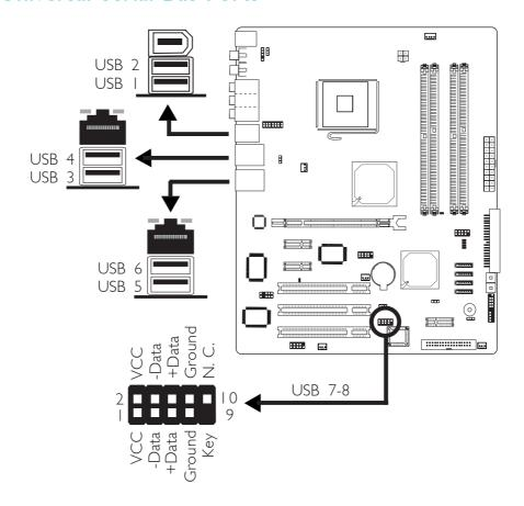
The system board supports 8 USB 2.0/1.1 ports. USB allows data exchange between your computer and a wide range of simultaneously accessible external Plug and Play peripherals.
