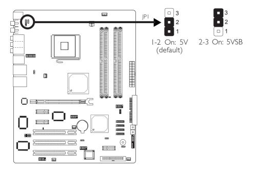
JPI is used to select the power of the PS/2 keyboard/mouse port. Selecting 5VSB will allow you to use the PS/2 keyboard or PS/2 mouse to wake up the system.
