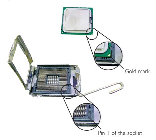
9. Insert the CPU into the socket until it is seated in place. The CPU will fit in only one orientation and can easily be inserted without exerting any force.
