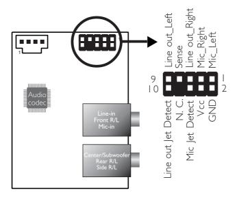
The front audio connector (J4) on the Karajan audio add-in card allows you to connect to the line-out and mic-in jacks that are at the front panel of your system. Using this connector will not disable the front right/left (line-out) and mic-in functions of the card. This is because the audio jacks on the Karajan audio card are 8 independent channels and they function independently from the front audio connector:
