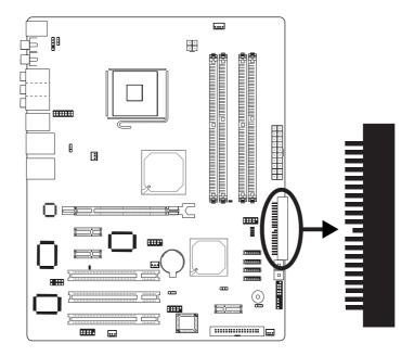
The system board is equipped with a 90° shrouded PCI IDE header that will interface two Enhanced IDE (Integrated Drive Electronics) disk drives. To prevent improper IDE cable installation, the shrouded PCI IDE header has a keying mechanism. The 40-pin connector on the IDE cable can be placed into the header only if pin I of the connector is aligned with pin I of the header.
