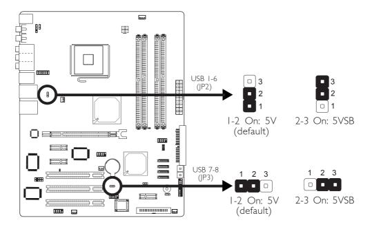
JP2 and JP3 are used to select the power of the USB ports. Selecting 5VSB will allow you to use the USB keyboard or USB mouse to wake up the system.
