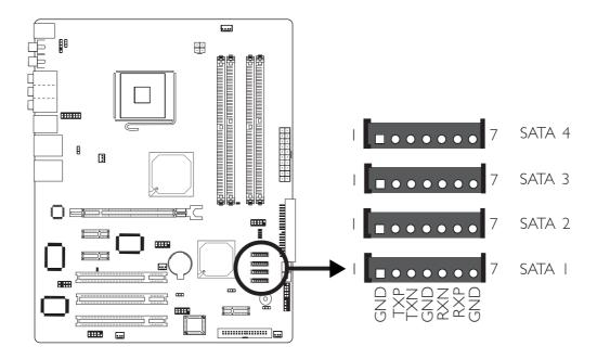
The system board is equipped with four Serial ATA connectors for connecting Serial ATA devices. Connect one end of the Serial ATA cable to J14 (SATA 4), J13 (SATA 3), J12 (SATA 2) or J11 (SATA 1) and the other end to your Serial ATA device.
