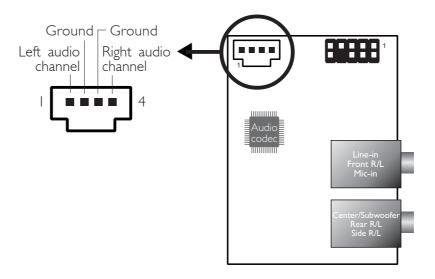
The CD-in (J2) connector on the Karajan audio add-in card is used to receive audio from a CD-ROM drive, TV tuner or MPEG card.
