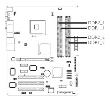
The system board supports two 240-pin DDR2 DIMM sockets and two 184-pin DDR1 DIMM sockets. Both types support dual channel.
