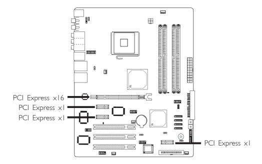
The system board allows installing one  $\times 16$  and three  $\times 1$  PCI Express cards.
