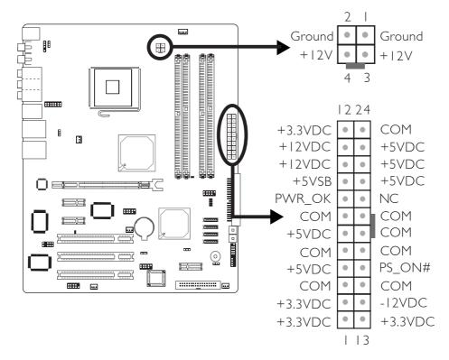
We recommend that you use a power supply that complies with the ATX12V Power Supply Design Guide Version I.I. An ATX12V power supply has a standard 24-pin ATX main power connector and a 4-pin +12V power connector that must be inserted onto CN11 and CN10 connectors respectively.
