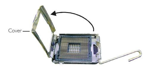
8. Position the CPU above the socket. The gold mark on the CPU must align with pin I of the CPU socket.
