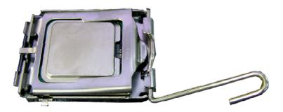
11. Push the lever down to lock the socket. The lever should hook onto the side tab to indicate that the CPU is completely secured in the socket.
