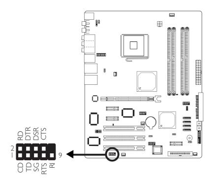
The system board is equipped with a COM connector (Teal/Turquoise) at location J4 of the system board for connecting an external serial port. It is a RS-232C asynchronous communication port with I6C550A-compatible UART that can be used with a modem, serial printer, remote display terminal or other serial devices.
