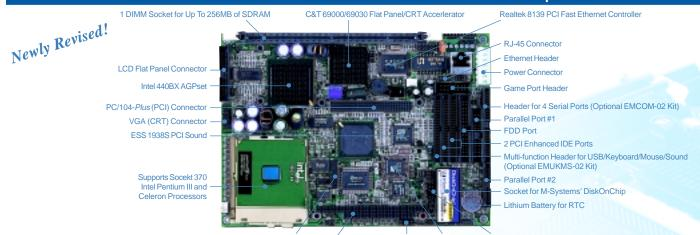
GPS Header (Optional EMGPS Kit) Digital I/O Header Flash BIOS IrDA Header PC/104-Plus (ISA) Connector
