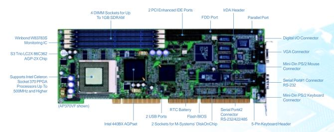
The AP370VF/F is a full-size PICMG Single Board Computer (SBC) that builts on the **Intel 440BX AGPset** and accepts Intel **Celeron Socket 370** PPGA processors up to 500MHz and higher. This gives you near Pentium II level performance with less heat build up and a lower cost.
