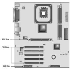
PCI Slots PCI slots are used to install expansion cards that have the 32-bit
