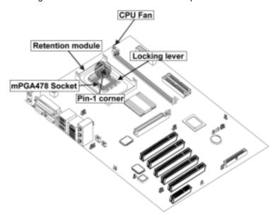
**Note:** The pin-1 corner is marked with an arrow ✓
