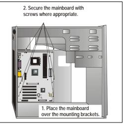
Ensure that your case has an I/O template that supports the I/O ports and expansion slots on your mainboard.
