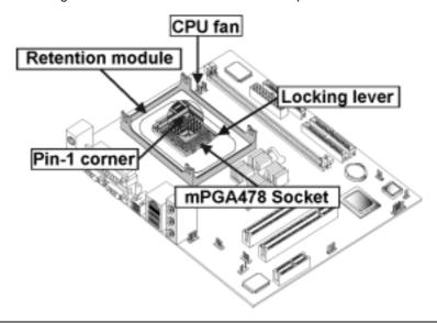
**Note:** The pin-1 corner is marked with an arrow **r**
