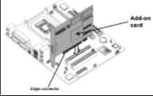
3. Secure the metal bracket of the card to the system case with a screw.
