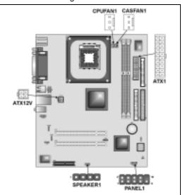
Note: When the system is heavily loaded, you should install, at a minimum, an ATX12V power supply with a 300W capacity.
