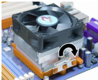
2. Make sure the CPU fan is plugged to the CPU fan connector. Please refer to the CPU cooling fan user's manual for more detail installation procedure.
