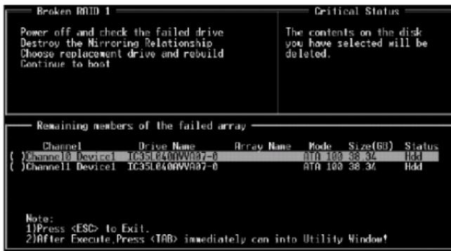
Highlight the target hard drive and press <Enter>, a warning message will appear. Press **Y** to use that hard drive to rebuild, or press **N** to cancel. Please note selecting option **Y** will destroy all the data on the selected hard drive.
