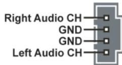
Connect other device (such as PCI TV Tuner audio out) to the connector.
