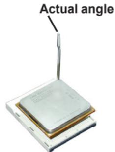
**Warning:** If the CPU does not fit, please change the insert orientation. Do not force the CPU into the socket.
