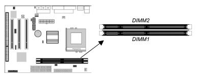
For this mainboard, you must use 168-pin, 3.3V unbuffered PC100 or PC133 SDRAM memory modules. You can install any size memory module from 32 MB to 512 MB, so the maximum memory size is  $2 \times 512$  MB = 1 GB.
