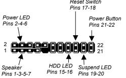
See the illustration below for a guide to the header pin assignments. Reset Switch Pins 17-18
