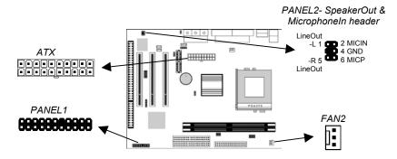
Connect the power connector from the power supply to the **ATX** connector on the mainboard.
