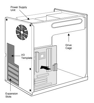
The illustration below shows the mainboard installing into a tower-type case.
