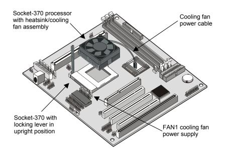
The mainboard must be configured to deliver the correct clock speed and the correct system bus for the kind of processor that you have installed. You can do this by using the system setup utility. The first time you start the system, immediately enter the setup utility and make the appropriate settings. Usually, you can automatically configure the CPU by using the CPU & BIOS Features page of the setup utility. See Chapter 3 for more information.
