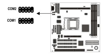
The serial ports extension bracket is supplied with this mainboard.
