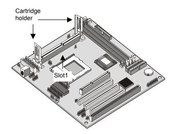
If the cartridge holder is not already installed, install it onto the slot1. Some cartridge holders are in two parts, one part for each end of the slot1. Other cartridge holders are a single assembly that sits over the whole length of the slot1.
