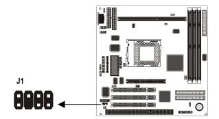
The digital audio extension bracket is an optional item. The digital audio extension bracket has an SPDIF-In jack, an SPDIF-Out jack, and Line-in jack.
