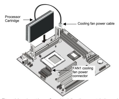
The mainboard must be configured to deliver the correct clock speed and the correct system bus for the kind of processor that you have installed. You can do this by using the system setup utility. The first time you start the system, immediately enter the setup system and make the appropriate settings. Usually, you can automatically configure the CPU by using the BIOS Features page of the setup utility. See Chapter 3 for more information.
