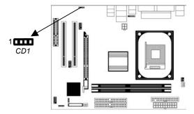
When you first start up your system, the BIOS should automatically detect your CD-ROM/DVD drive. If it doesn't, enter the Setup Utility and configure the CD-ROM/DVD drive that you have installed. On the mainboard, locate the 4-pin connector **CD1**.
