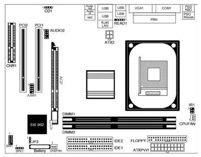
**Note:** Any jumpers on your mainboard not appearing in the illustration above are for testing only.
