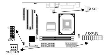
Connect the power connector from the power supply to the **ATXPW1** connector on the mainboard. **ATX2** is the CPU Vcore power connector.
