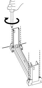
7. Horizontally slide the Heatsink Top Support into the lowest gaps on the CPU module heatsink as shown below.
