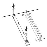
4. Install two Retention Mechanism Attachment Mounts on the board
