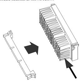
8. Slide the CPU module into the Retention Mechanism Assembly.
