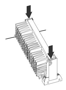
10. Hook the Heatsink Top Support to the Heatsink Support Base to affix the CPU module.
