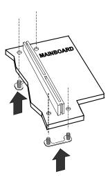
5. Place the Retention Mechanism Assembly on the board, on top of the Rentention Mechanism Attachment Mounts.
