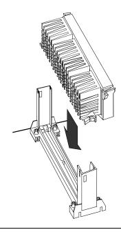
9. Press the buttons on either end of the CPU module.
