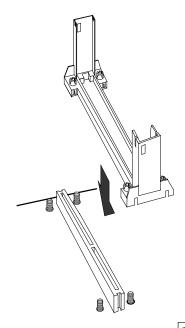
6. Affix the Retention Mechanism Assembly with four screws.
