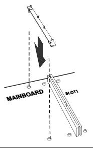
3. Affix it by inserting one "T"-shaped plastic plug into the hole on each end
