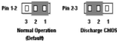
Figure 2-8. CCMOS1 jumper setting
