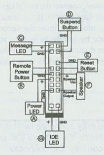
Power LED (A): (2-pin male) The system power LED lights when the system is powered on.
