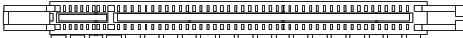
Mazarine PCI Express x16 Slot (PCI_EX1) supports up to PCI Express 2.0x16 speed
