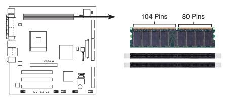
K8S-LA 184-pin DDR DIMM sockets
