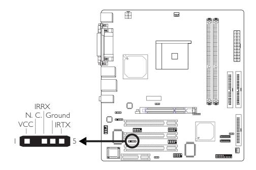
Connect your IrDA cable to connector J5 on the system board.
