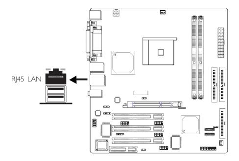
The system board is equipped with an onboard RJ45 fast-ethernet LAN port at location CN5 of the system board. It allows the system board to connect to a local area network by means of a network hub.
