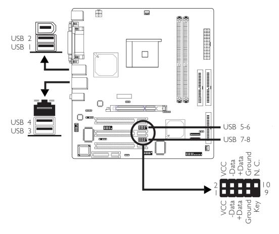
Four onboard USB 2.0/1.1 ports (Black) are at locations CN6 (USB 1-2) and CN5 (USB 3-4) of the system board.
