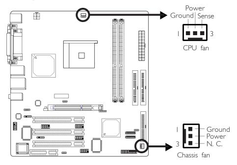
Connect the CPU fan's cable connector to the CPU fan connector (J20) on the system board. The chassis fan connector (J10) is used to connect an additional cooling fan. The cooling fans will provide adequate airflow throughout the chassis to prevent overheating the CPU and system board components.
