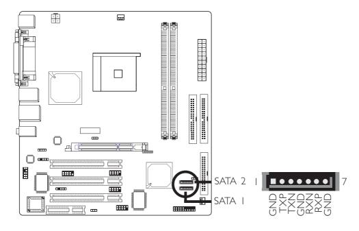
Connect one end of the Serial ATA cable to JI5 (SATA 2) or JI6 (SATA I) and the other end to your serial ATA device.
