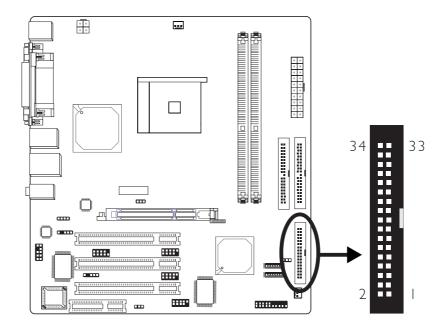
The system board is equipped with a shrouded floppy disk drive connector for connecting two standard floppy disk drives. To prevent improper floppy cable installation, the shrouded floppy disk header has a keying mechanism. The 34-pin connector on the floppy cable can be placed into the header only if pin I of the connector is aligned with pin I of the header.
