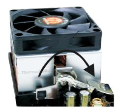
6. Connect the CPU fan's cable connector to the CPU fan connector on the system board.
