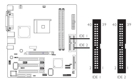
The system board is equipped with two shrouded PCI IDE headers that will interface four Enhanced IDE (Integrated Drive Electronics) disk drives. To prevent improper IDE cable installation, each shrouded PCI IDE header has a keying mechanism. The 40-pin connector on the IDE cable can be placed into the header only if pin I of the connector is aligned with pin I of the header.
