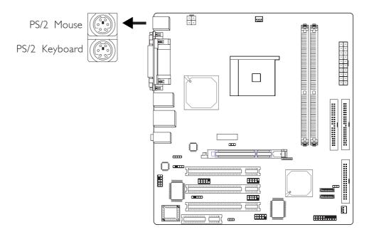
The system board is equipped with an onboard PS/2 mouse (Green) and PS/2 keyboard (Purple) ports - both at location CNI of the system board. The PS/2 mouse port uses IRQ12. If a mouse is not connected to this port, the system will reserve IRQ12 for other expansion cards.
