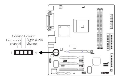
The CD-in (J2) connector is used to receive audio from a CD-ROM drive, TV tuner or MPEG card.
