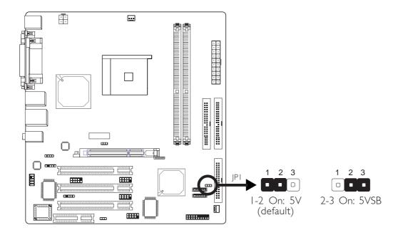
JPI is used to select between 5V and 5VSB power. Selecting 5VSB will allow you to use a PS/2 keyboard, PS/2 mouse or a USB device to wake up the system.
