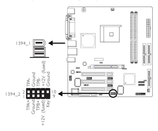
The system board is equipped with an onboard IEEE 1394 port at location CN6 (IEEE 1394\_I) of the system board.
