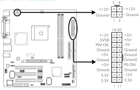
Use a power supply that complies with the ATX12V Power Supply Design Guide Version 1.1. An ATX12V power supply has a standard 20-pin ATX main power connector and a 4-pin +12V power connector that must be inserted onto CN9 and CN8 connectors respectively.
