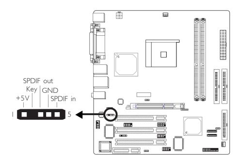
The S/PDIF-in/out connector (J4) is used to connect external S/PDIF ports. The S/PDIF ports may be mounted on a card-edge bracket. Install the card-edge bracket to the system chassis then connect the audio cable connector to J4. Make sure pin 1 of the audio cable connector is aligned with pin 1 of J4.
