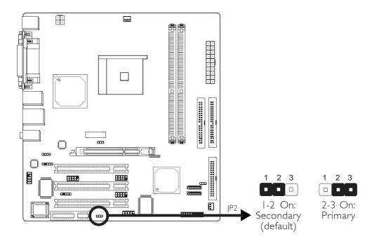
CNR cards are defined as primary and secondary. Set this jumper according to the type (primary or secondary) of CNR card installed in the CNR slot.
