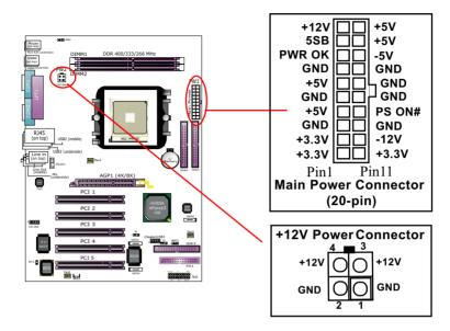
To set up Power Supply on this mainboard:
