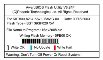
(5) When the process is complete, remove the Floppy Diskette and press F1 to restart the system to put the new BIOS into effect.
