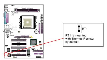
Thermal Resistors RT1: A thermal resistor is mounted by default to connector RT1 so as to detect the temperature of the chassis. What RT1 does is to transmit the thermal signal to Hardware Monitor.
