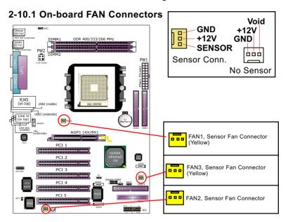
Both Sensor and No-sensor Fan Connectors support CPU/AGP/System/Case cooling fan with +12V mode. A Hardware Monitor chipset is on board, with which user can install a Hardware Monitor Utility and read the fan speed transmitted from the sensor fan connector. Otherwise, user can read the fan speed from the "Hardware Monitor Status" via CMOS BIOS.
