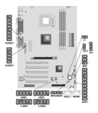
**LAUDIO1: Front panel audio header**This header allows the user to install auxiliary front-oriented microphone and line-out ports for easier access.
