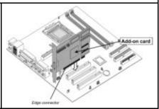
3. Secure the metal bracket of the card to the system case with a screw.
