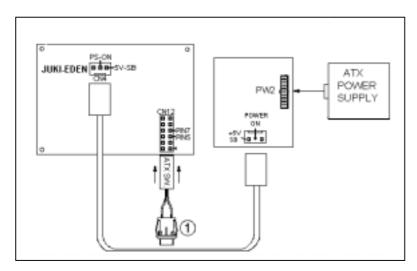
Connect the ATX power button switch to the CN12 (power button). And connect the power cable from Backplane to CN4 of CPU card.
