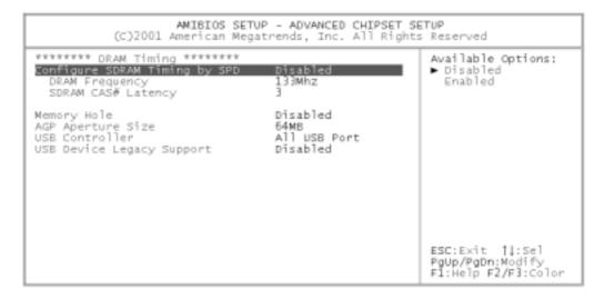
This section enables you to configure the system based on the specific features of the installed chipset. The chipset manages bus speeds and access to system memory resources, such as DRAM and the external cache. It also coordinates communications between the conventional ISA bus and the PCI bus. Do not change the default settings or it may cause system malfunction.
