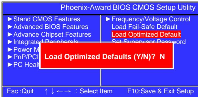
Pressing '**Y**' loads the default values that are factory settings for optimal performance system operations.
