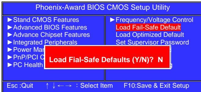
Pressing '**Y**' loads the BIOS default values for the most stable, minimal-performance system operations.
