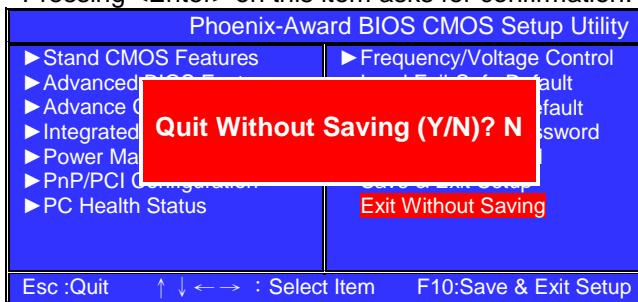
This allows you to exit Setup without storing in CMOS any change. The previous selections remain in effect.
