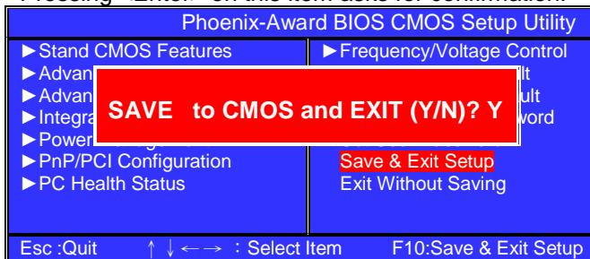
Pressing “Y” stores the selections made in the menus in CMOS – a special section of memory that stays on after you turn your system off. The next time you boot your computer, the BIOS configures your system according to the Setup selections stored in CMOS. After saving the values the system is restarted again.
