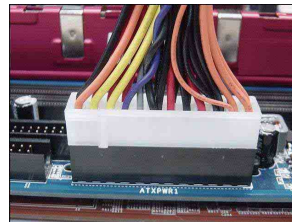
Plugged from a 24-pin ATX12V power.
