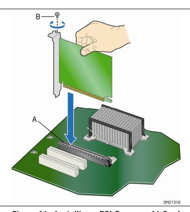
Figure 16. Installing a PCI Express x16 Card
