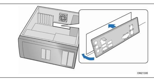
Figure 4. Installing the I/O Shield
