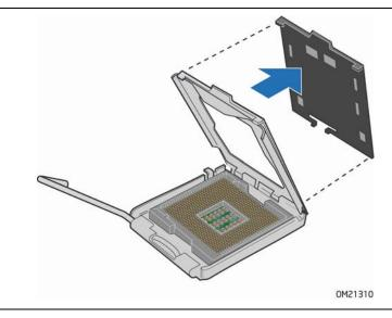
Figure 8. Remove the Protective Socket Cover
