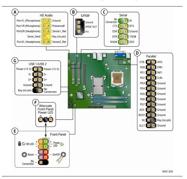
Figure 20. Internal Headers and Connectors
