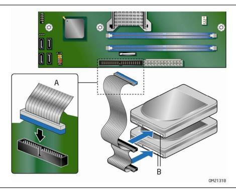
Figure 18. Connecting the IDE Cable
