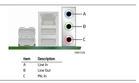
Figure 21. Back Panel Audio Connectors
