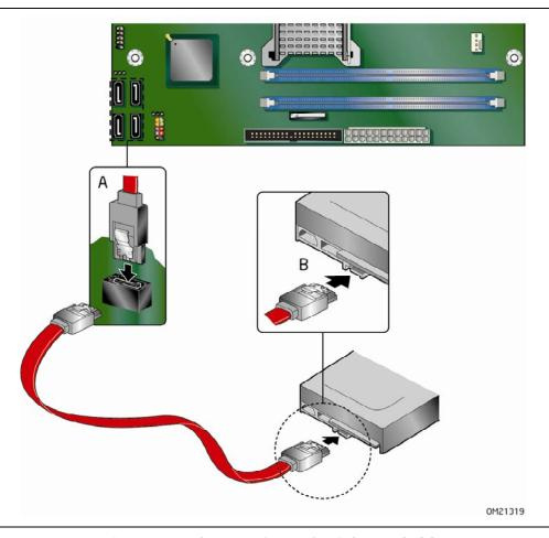
Figure 19. Connecting a Serial ATA Cable
