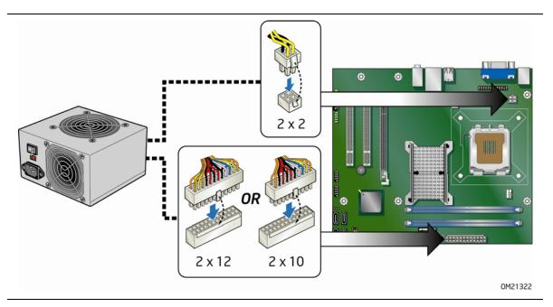
Figure 23. Connecting Power Supply Cables
