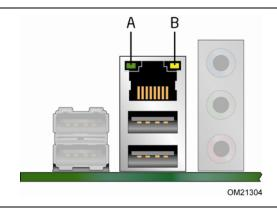
Figure 2. LAN Connector LEDs
