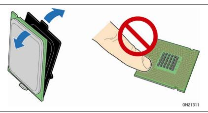
Figure 9. Remove the Processor from the Protective Processor Cover
