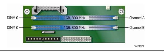
Figure 13. Dual Channel Memory Configuration Example
