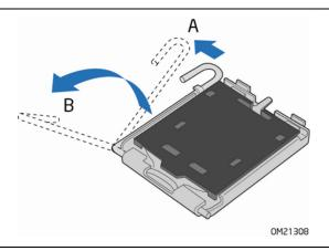
Figure 6. Lift the Socket Lever
