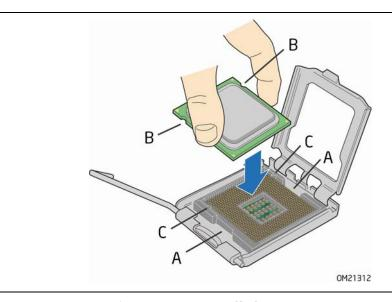
Figure 10. Install the Processor
