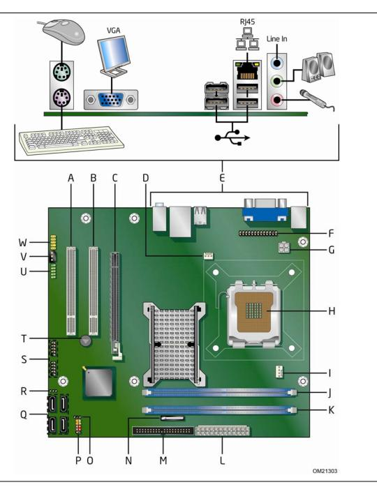
Figure 1. Intel Desktop Board DG41RQ Components
