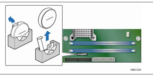
Figure 25. Removing the Battery
