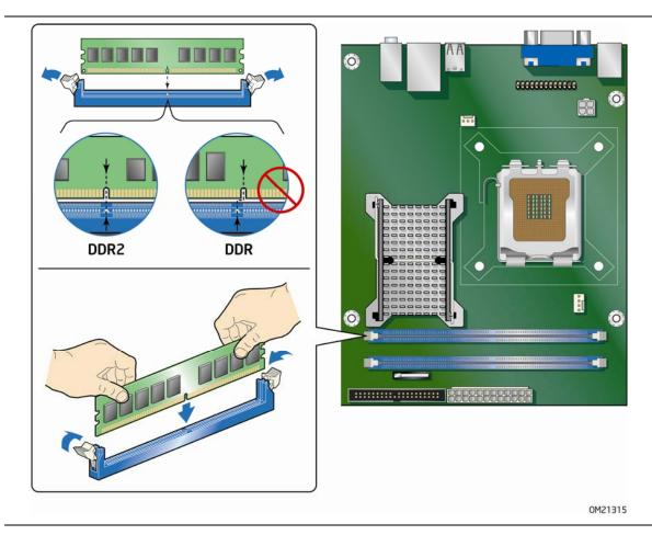
Figure 15. Installing a DIMM
