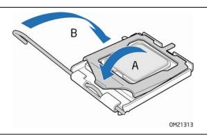
Figure 11. Close the Load Plate
