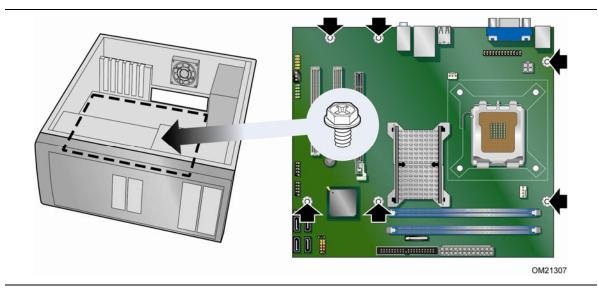
Figure 5. Intel Desktop Board DG41RQ Mounting Screw Hole Locations
