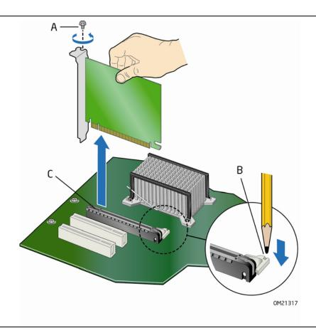
Figure 17. Removing a PCI Express x16 Card
