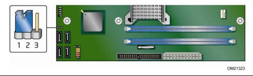
Figure 24. Location of the BIOS Configuration Jumper Block
