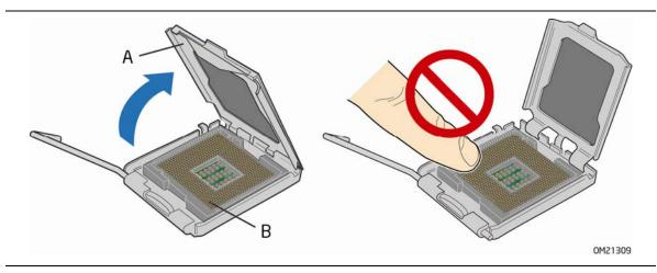
Figure 7. Lift the Load Plate
