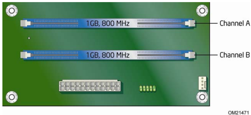
Figure 14. Dual Channel Memory Configuration Example
