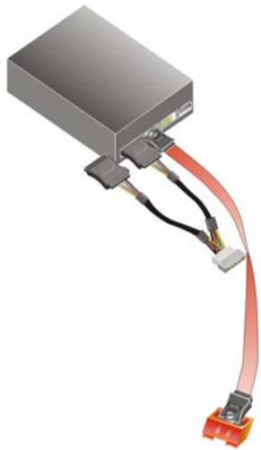
Figure 5-19: SATA Power Drive Connection
