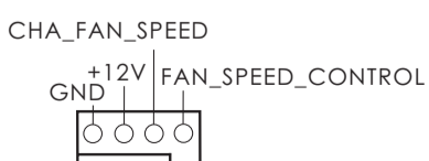
7 : 4-Pin Chassis FAN Connector (+12V)
