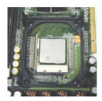
**STEP4:** Attach the heat sink onto the CPU and close the levers to fix the attachment.
