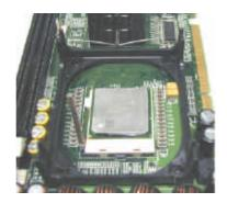
**STEP3:** Push the lever down to close the socket.
