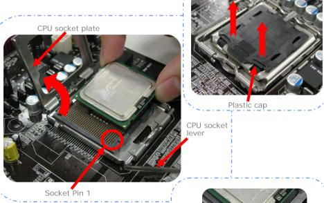
Warning: If you do not match the CPU socket Pin 1 and CPU golden arrow well, you may damage the CPU. And please don't touch CPU socket pins when installing CPU.
