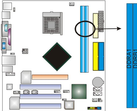
1. Unlock a DIMM slot by pressing the retaining clips outward. Align a DIMM on the slot such that the notch on the DIMM matches the break on the Slot.
