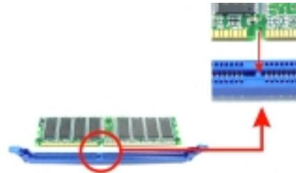
2. Insert the DIMM vertically and firmly into the slot until the retaining chip snap back in place and the DIMM is properly seated.
