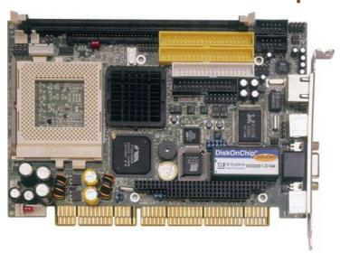
The HS-6251 is a 133MHz FSB, VIA VT8606 chipset-based, PCI-ISA Bus Celeron<sup>TM</sup>/Coppermine<sup>TM</sup>/Tutalatin<sup>TM</sup> CPU SBC. With features such as enhanced I/O effects with CRT/Panel, LAN and audio interface all combined, the HS-6251 is an ideal all-in-one Industrial Single Board Computer for the demanding embedded applications.
