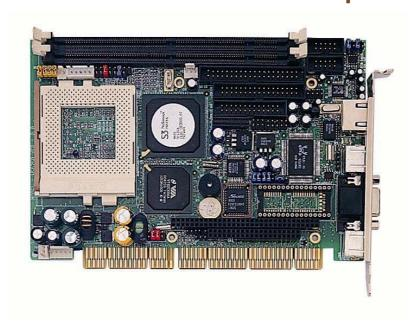
The HS-6250 is a 133MHz FSB, VIA VT8605 chipset-based, PCI-ISA Bus Celeron<sup>TM</sup>/Coppermine<sup>TM</sup>/Tutalatin<sup>TM</sup> CPU SBC. With features such as enhanced I/O effects with CRT, LAN and audio interface all combined, the HS-6250 is an ideal all-in-one Industrial Single Board Computer for the demanding embedded applications.
