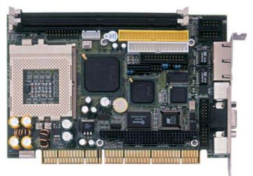
The HS-6238 is a 133MHz FSB Intel<sup>®</sup> 82815 chipset-based board designed for PCI-ISA Bus Celeron™/Coppermine™/Tualatin™ 800MHz~1.2GHz CPU compatibility. These features combine and make the HS-6238 an ideal all-in-one industrial single board computer. Additional features include an enhanced I/O with 4COM ports, Dual LAN and CRT/Panel interface.
