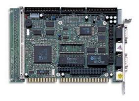
The HS-3100 is ISA Bus ALi M6117C chipset industrial single board computer. The board design combine together with all necessary input and output effects interfaces which makes it an ideal all-in-one industrial single board computer. The board design with 40MHz Bus clock rate architecture. The HS-3100 supports one SIMM socket with a max. capacity of 16MB and 4MB RAM onboard.
