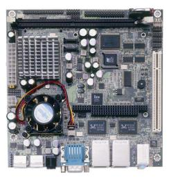
The HS-1770 is a VIA CX700(M) chipset-based board designed. The HS-1770 is an ideal all-in-one mITX board. Additional features include an enhanced I/O with CF, CRT/LVDS, TV-Out, dual LAN, audio, SPDIF, SATA, 4 COM, USB2.0, and PC/104 interfaces.
