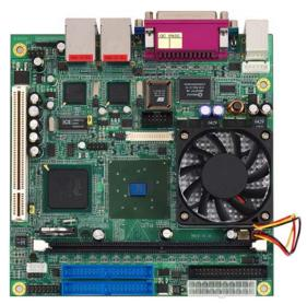
The HS-1746 is an Intel<sup>®</sup> 855GME GMCH/ICH4 chipset-based board designed mITX board. Intel<sup>®</sup> Pentium<sup>®</sup> M/Celeron<sup>®</sup> M processor 1.3~2.0GHz compatibility. The combination of these features makes the HS-1746 an ideal all-in-one industrial mITX board. Additional features include an enhanced I/O with CRT/LVDS Panel, dual Giga LAN, audio, COM, IrDA and USB2.0 port interface.
