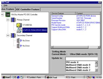
10. Once you select the IDE Controller Feature from the IDE Tool dialog box, a list of read-only information related to the system's IDE controller is shown.
