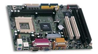
The HS-1000 is a VIA VT8601T chipset-based board designed with Socket 370 for Intel® Celeron™/Coppermine™/Tualtain™ 633MHz~ 1.3GHz CPU. These features combine and make the HS-1000 an ideal industrial ATX motherboard. Additional features include an enhanced I/O with CRT, audio, and game port interface.
