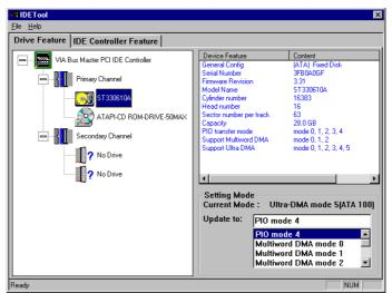
9. The Drive Feature dialog box has 2 columns of information. The left column lets you to view the hardware installed on your system. When you select any hardware, the right column displays the device's information and specifications. You may also update the settings of your devices from the right column.
