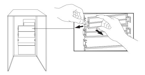
Installing a Hard Disk Drive in a Front-Access Shelf Unscrew and remove an unused drive tray. Mount the drive on the tray, sliding the drive into place, and securing it with four screws on the underside.
