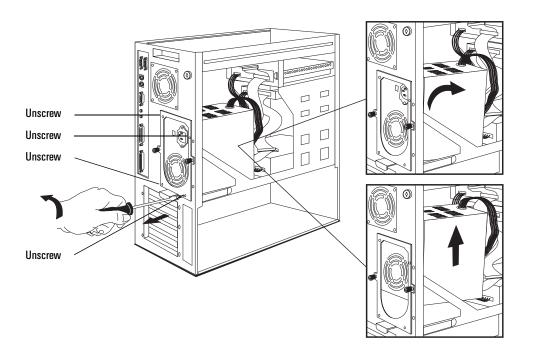
To install the new power supply, reverse the steps which were followed when removing the old power supply.
