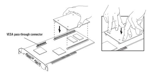
If you install a VESA-standard video accessory board that uses the MGA video adapter, connect the accessory board's cable to the VESA pass-through connector on the MGA adapter board.
