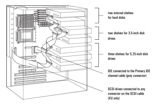
All models have an integrated IDE controller. All models of HP Vectra XU 6/ xxx PC have an integrated SCSI controller.
