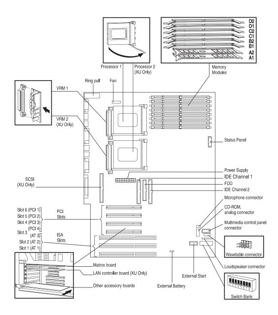
Installing the New System Board
