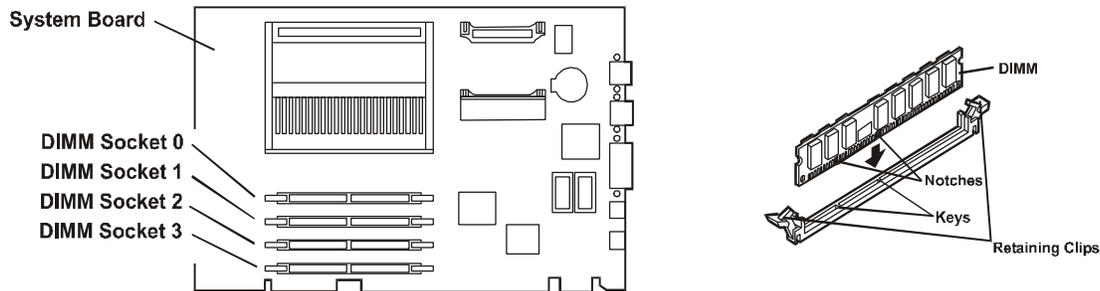
**CAUTION** Do not rock the DIMM into place, but apply firm and even pressure directly downward. If the retaining clips do not close, remove the module and repeat Steps 3 through 5.
