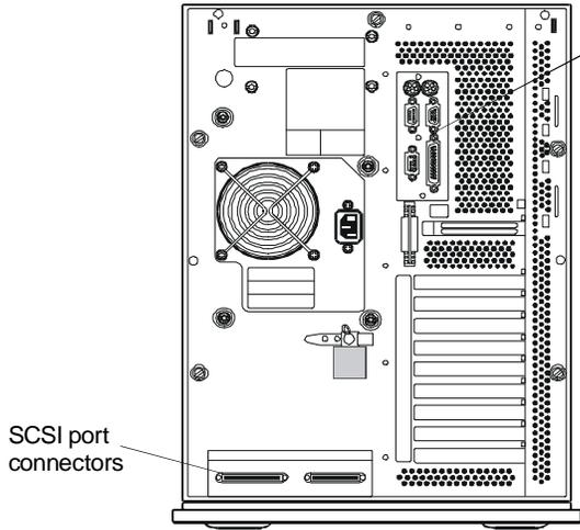
Keyboard, Mouse, serial, and display connectors
