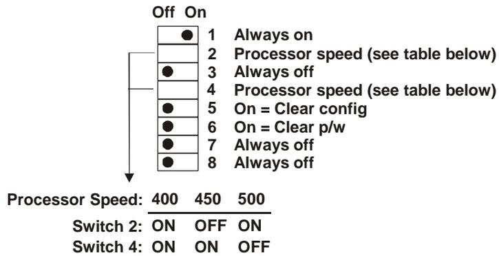
Note: Only processor speeds for the 100 MHz bus are supported.
