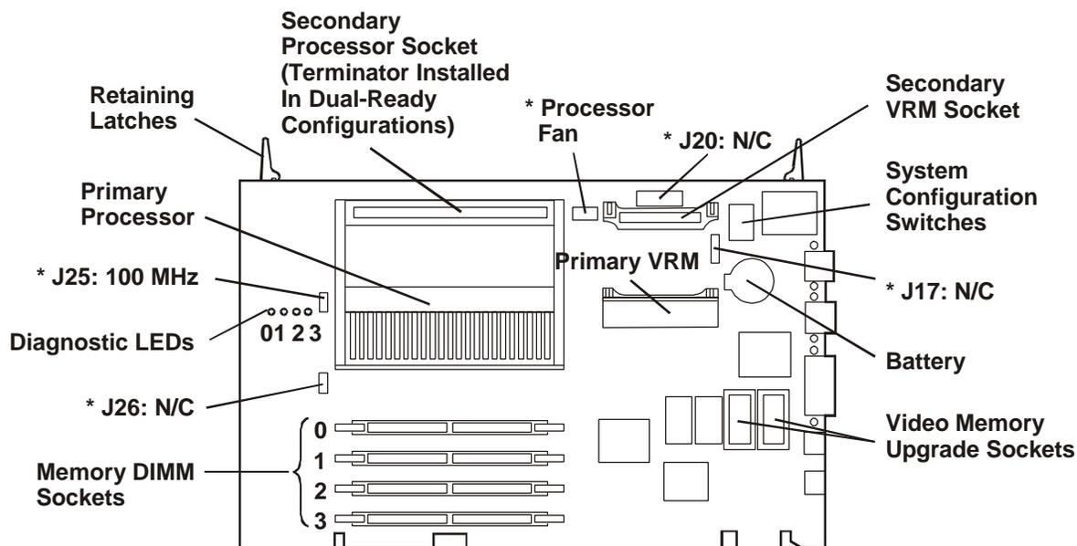
\* Cable connectors are labeled with function.
