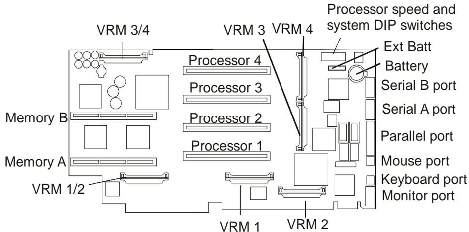
Note: Processor slots without processors have terminators.
