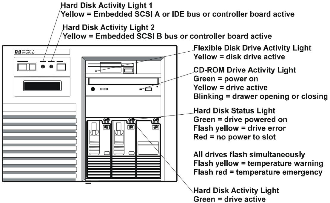
For some SCSI controller boards, you must connect the hard disk activity light.
