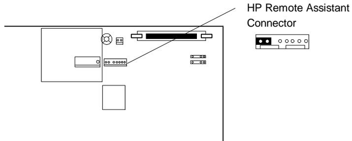
**WARNING** If the HP Remote Assistant is not installed and there is no jumper on PS REMOTE and PS ON, the system will NOT power up.
