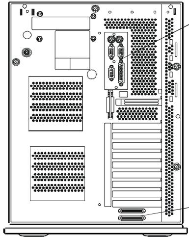
Keyboard, Mouse, serial, and display connectors
