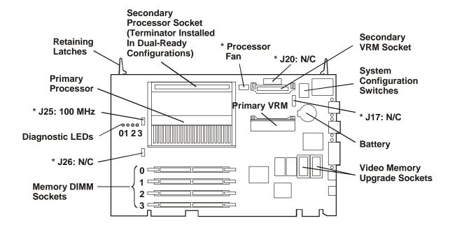
\* Cable connectors are labeled with function.
