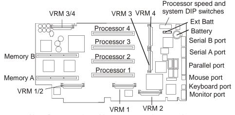
Note: Processor slots without processors have terminators.
