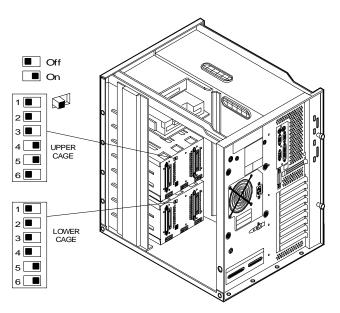
The switch 6 setting determines upper and lower cage functionality. Switches 1 and 2 are always set to Off.
