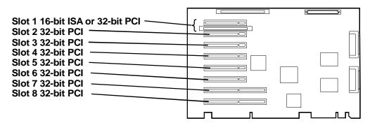
Boot order for PCI controllers is determined by slot location. The system searches for a bootable device in the following order:
