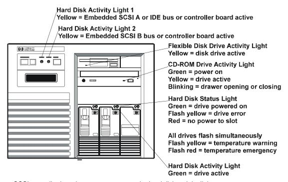
For some SCSI controller boards, you must connect the hard disk activity light.
