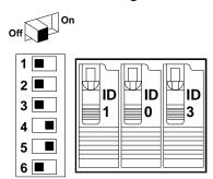
This is the default SCSI switch setting for this configuration. SCSI ID 2 is reserved for an optional DAT (Digital Audio Tape) drive that can be installed in upper shelf 3 or 4. The standard CD-ROM drive is shipped with SCSI ID 5.
