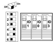
This is the default SCSI switch setting for this configuration. SCSI ID 2 is reserved for an optional DAT (Digital Audio Tape) drive that can be installed in upper drive tray 3 or 4. The standard CD-ROM drive is shipped with SCSI ID 5.
