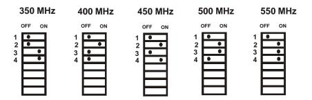
NOTE: Only the first 4 switches set the processor clock.
