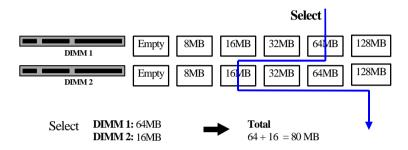
To select 1 out of 6 items (empty, 8MB, 16MB, 32MB, 64MB, 128MB) in DIMM1. Then, repeat again in DIMM2 to go through your own path.
