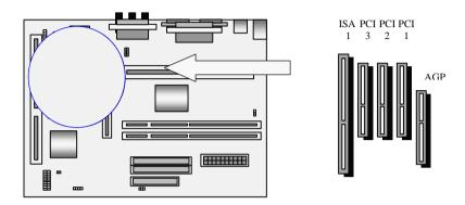
This motherboard contains 5 expansion slots onboard. One 16-bit ISA Bus, Three 32-bit
