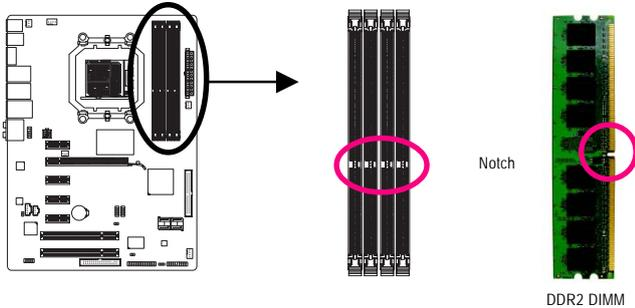
A DDR2 memory module has a notch, so it can only fit in one direction. Follow the steps below to correctly install your memory modules in the memory sockets.
