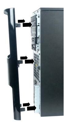
**2** Press the bezel firmly into place.
