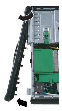
**3** Swing the bottom of the bezel out until the top of the bezel can be disengaged from the top of the computer, then remove the bezel.
