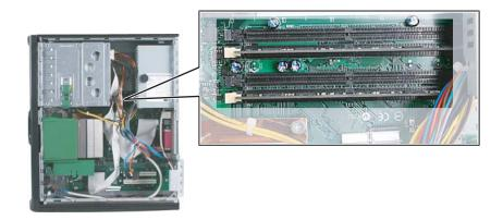
**5** If you are removing a DIMM from the memory module bank, gently pull the plastic tabs away from the sides of the memory module and remove it.
