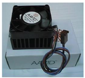
Figure 3:Boxed Celeron<sup>™</sup> Socket370 Processor & Heat sink support
