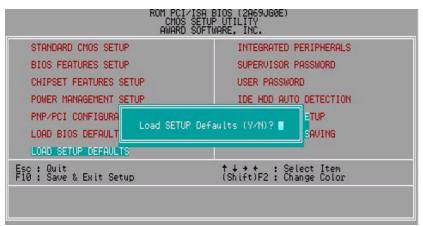
Figure 4.8: Load Setup Defaults
