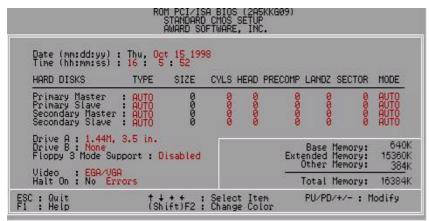
Figure 4.2: Standard CMOS Setup Menu
