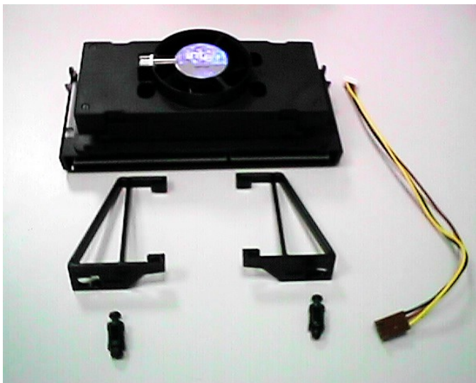
Figure 4:Boxed Pentium® II Processor & Heat sink support
