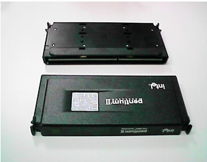
Figure 2:OEM Pentium® II Processor
