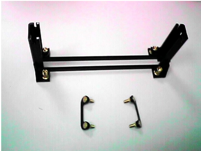
Figure 1:Retention Mechanism & attach Mount
