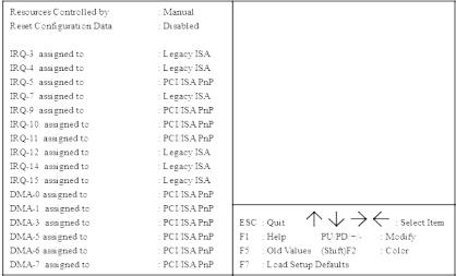
Figure 4.6: PCI Slot Configuration
